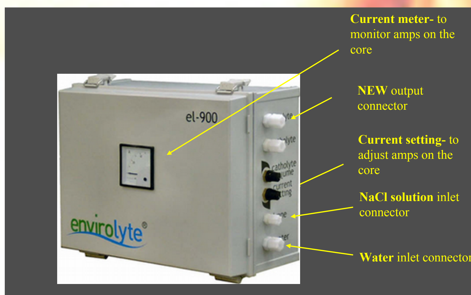
Figure 2. Neutral electrolyzed water generator
